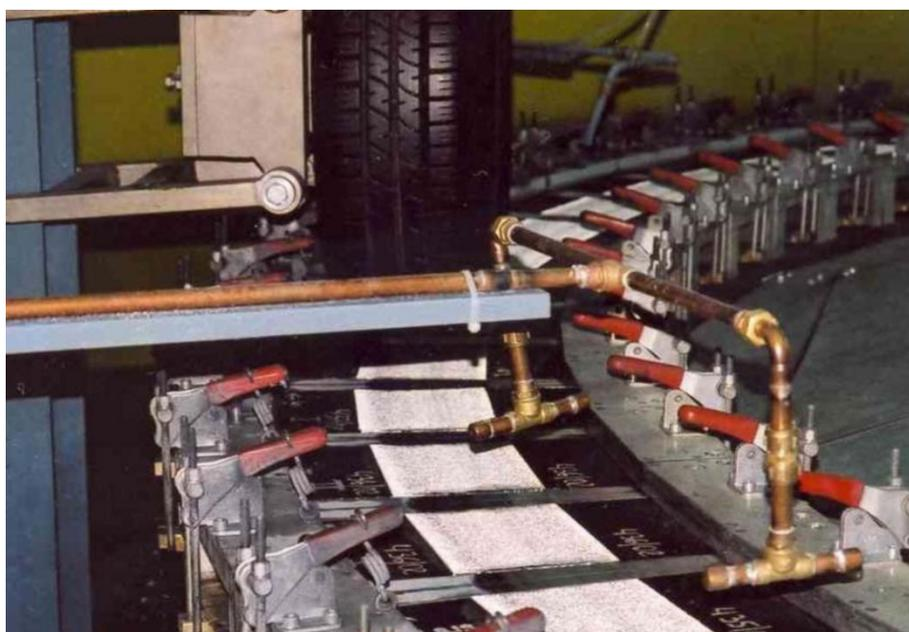
***Figure 4: AETEC turntable detail: wheel on paint test panels***
