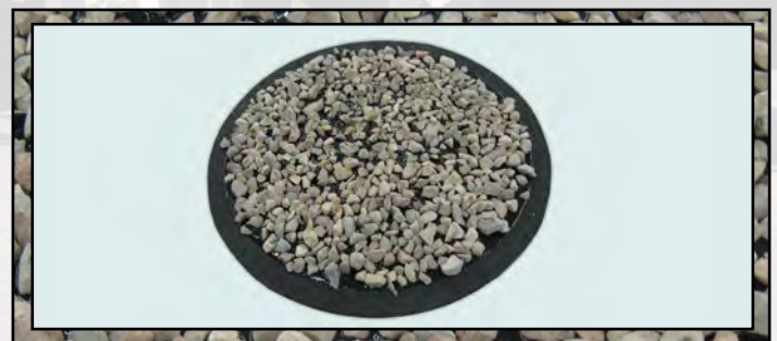
Figure 2 - Kraton D1192-Modified CRS-2P Emulsion Sweep Test Pad - Post-Sweep
