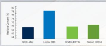
Kraton D1192 and Kraton D0243-modified CRS-2P emulsions can be produced at low residue content
