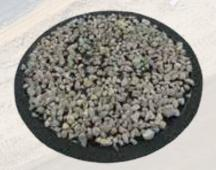
Figure 2 - Kraton D1192-Modified CRS-2P Emulsion Sweep Test Pad - Post-Sweep
