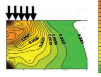
Kraton HiMA [150mm (6") asphalt] Total damage at 9000 axle loads
