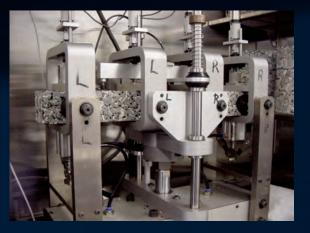
30/50 pen bitumen with 7.5% Kraton D0243 in 22 mm mix Full sine loading, 8Hz, 20 °C 100x load cycles same micro-strain HIGHLY MODIFIED ASPHALT (HIMA) NEXT GENERATION IN ASPHALT PAVEMENT DESIGN
