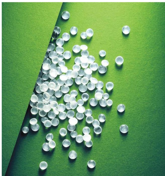
New rosin ester technology enabled by a novel catalyst class allows for the production of near water-white rosin esters.
